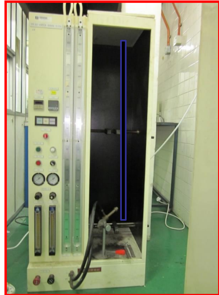
Vertical burning tester on single cable
