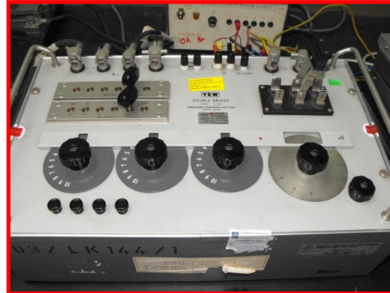
Conductor resistance test with Precision Double Bridge
