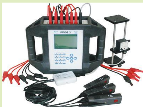
Portable Test Device used by ST for testing of electricity meters
