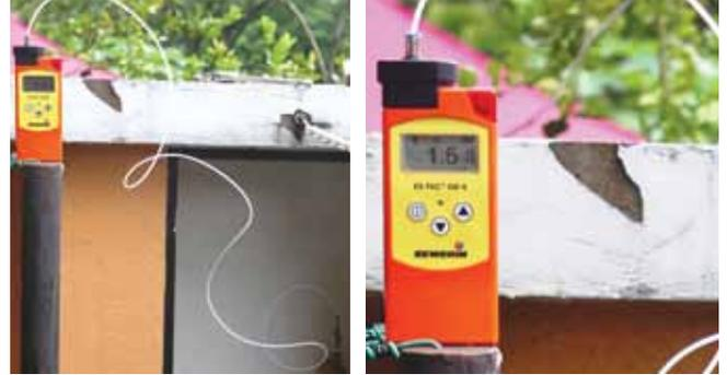
Odorant level measurement using Electrochemical Sensors and reading example
