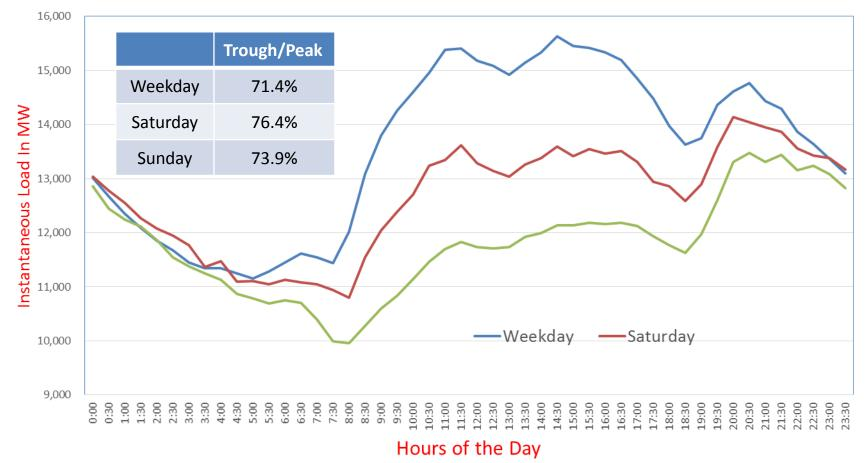
In Peninsular Malaysia Grid System, the ratio of trough vs peak demand is around 74%. In designing UFLS scheme, the quantum of load shed is based on peak load e.g. 55% of peak load. At other times, it is assumed that the load will be proportional (eg. 55%) to the system demand at that time
