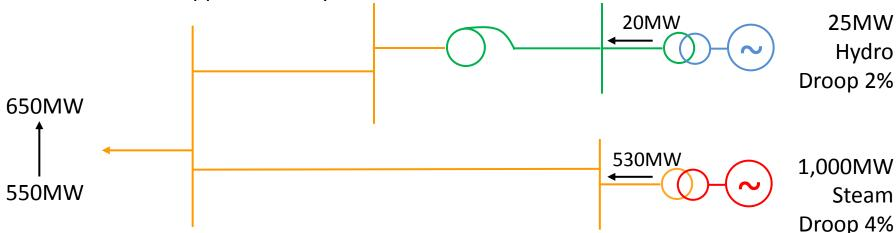
Hydro droop 2%: 1Hz change in frequency = 25MW change in output Steam droop 4%: 2Hz change in frequency =1,000MW change in output
