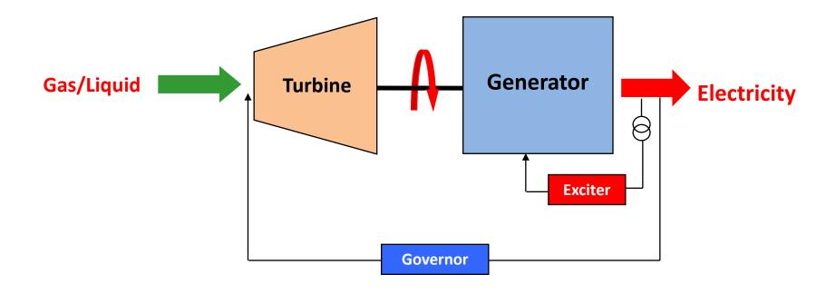
**Exciter** of a generator controls the voltage of a generator
