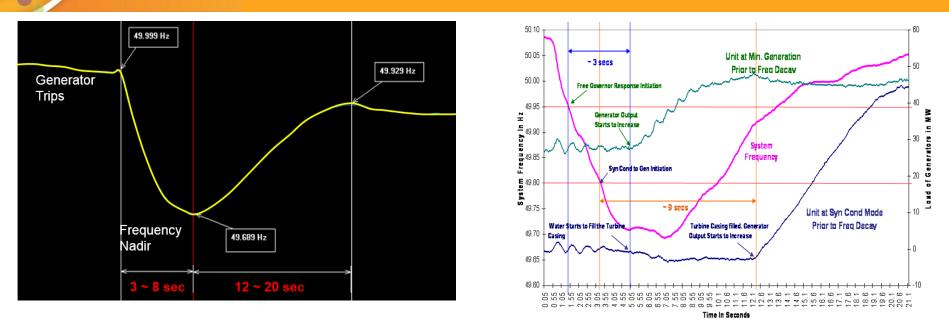
The objective is to restore system load/generation balance, stabilize the system frequency and prevent turbine blades from permanent damage.
