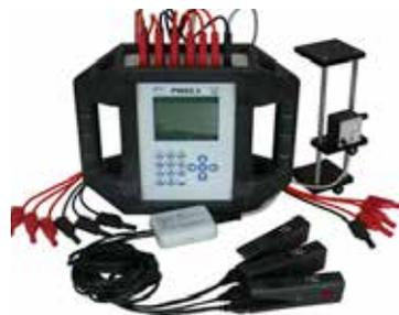
A portable tester used to test the accuracy of electricity meters on consumers' premises
