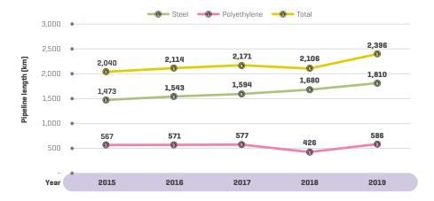
Figure 13: Length of Natural Gas Pipelines in Operation in the Peninsula
