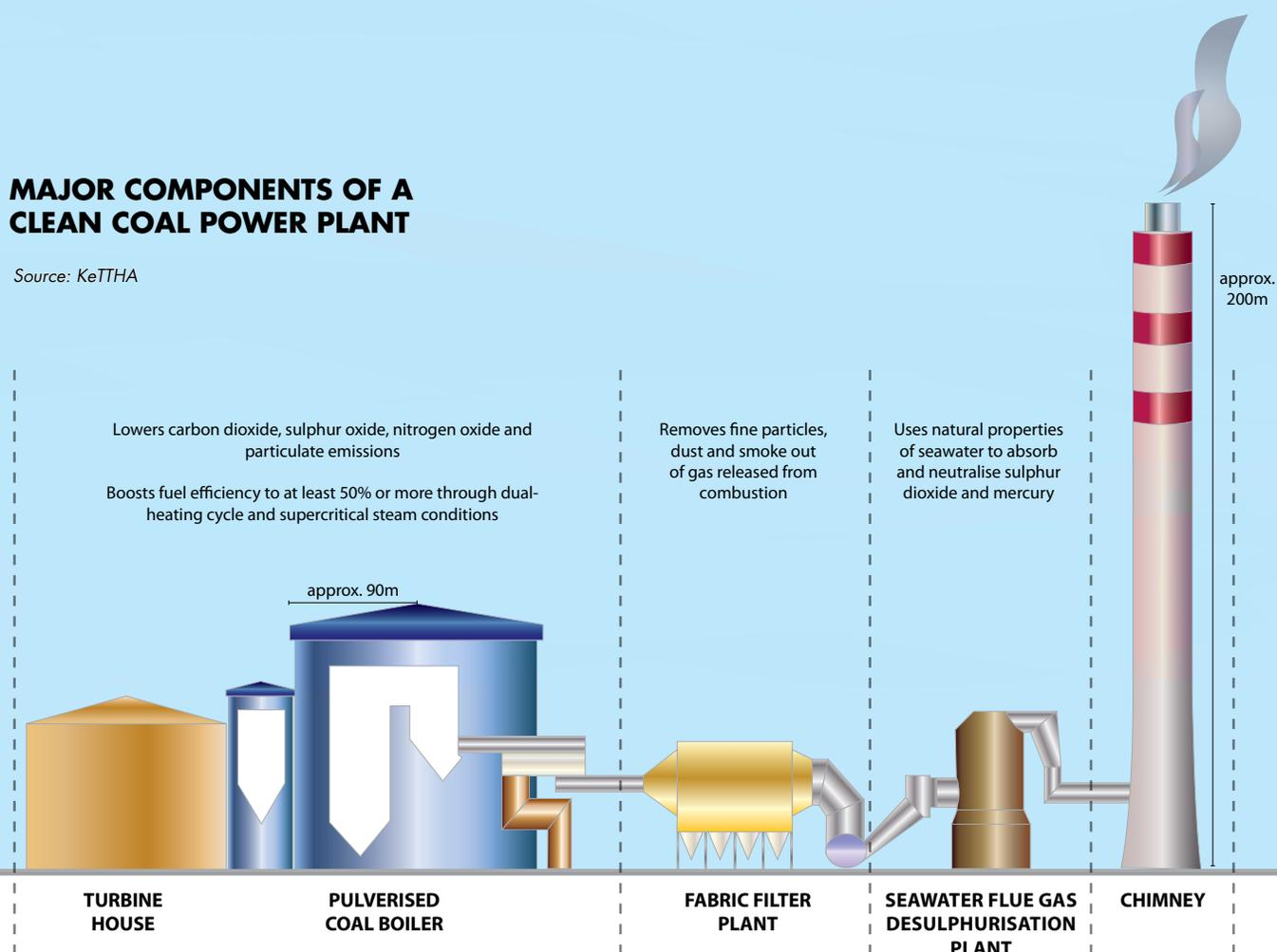
for its coal-fired boilers upon its completion in 2015, will generate 14% more power and remove up to 90% of sulphur oxide from the flue gas. This new 1,010MW project will provide additional capacity to power nearly 2 million Malaysian households while ensuring the environment is protected.
