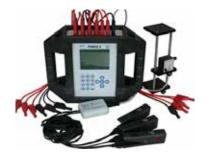
A portable tester used to test the accuracy of electricity meters on consumers' premises
