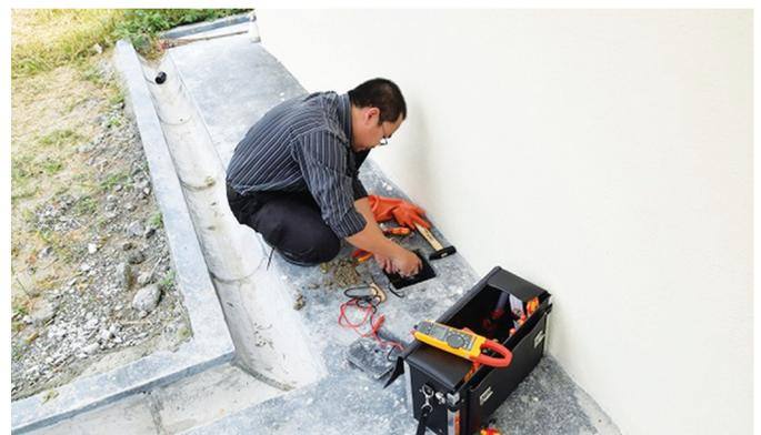
Testing insulation and earthing resistance in the investigation of a fatal accident case.
