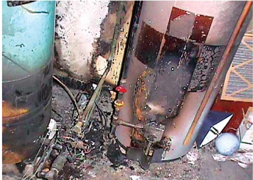
*An exploded water heater as a result of improper installation. The Energy Commission provides guidelines for proper and safe water heater installation to prevent accidents like these.*
