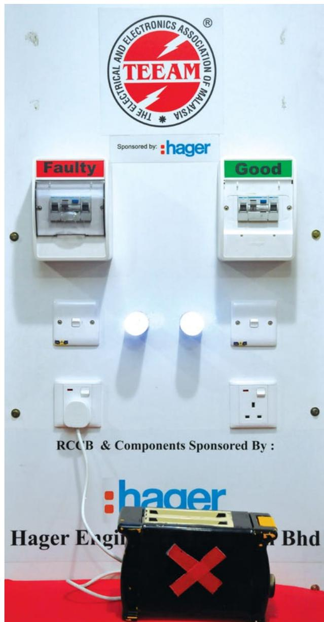
*TEEAM's portable demonstration setup includes a toaster, deliberately rigged to be faulty, that is plugged into a circuit with a functioning RCCB unit, and one with a malfunctioning unit. In the former circuit, the RCCB will trip the moment the toaster is switched on, saving the user from a nasty shock.*
