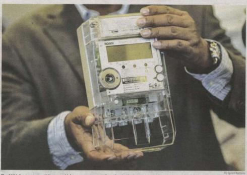
The AMI infrastructure architecture which uses smart meter allows for the device to communicate with the meter data management and head-end systems via the radio frequency mesh network
