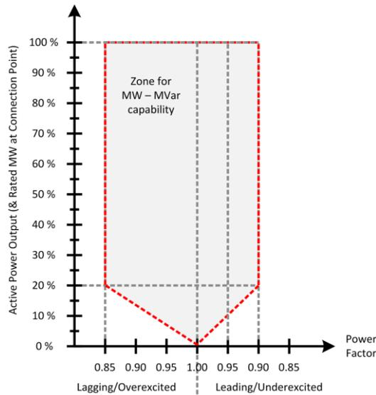
Fig. 6.1: Reactive power requirement at connection point
