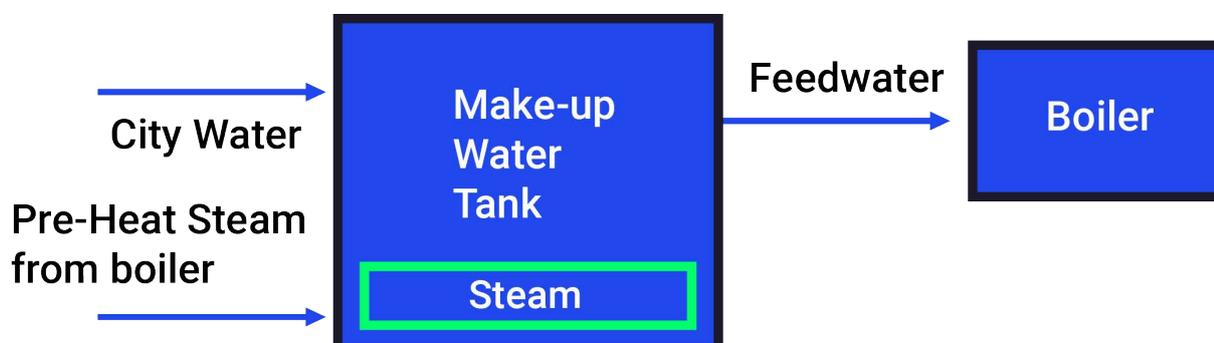
**Figure 4: Proposed boiler make-up water tank configuration**
