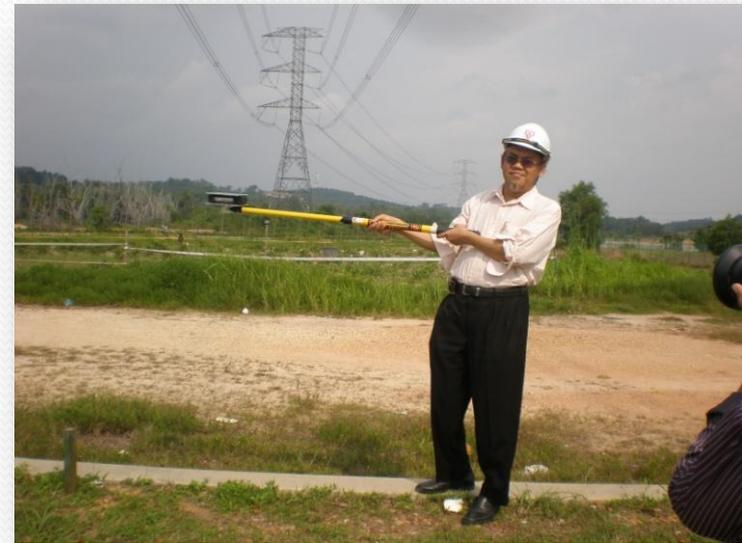
**Electric Field Measurement underneath the 500 kV Lines of Site 6**
