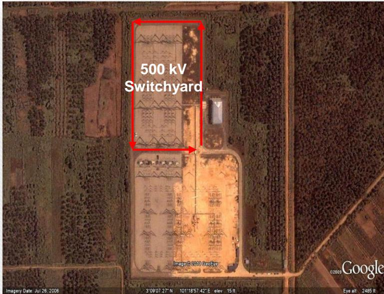
**Measurement Path for the Magnetic Field Measurement at the Perimeter of the 500 kV Switchyard of Site 5**
