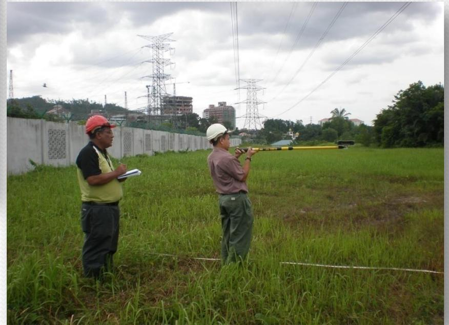
**Electric and Magnetic Field Measurements Conducted Underneath the Transmission Lines**
