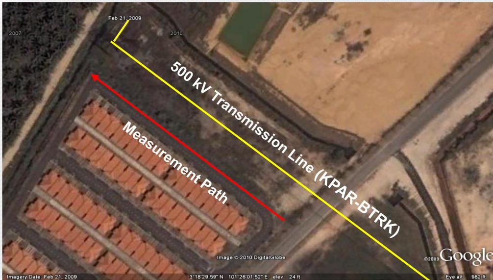
Magnetic Field Longitudinal Profile Measurement
