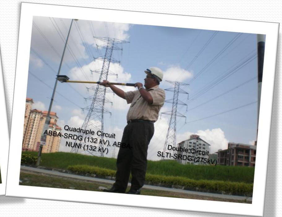
**Electric and Magnetic Field Measurements Conducted Underneath the Transmission Lines**
