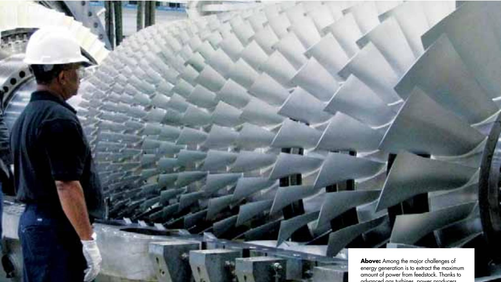
**Above:** Among the major challenges of energy generation is to extract the maximum amount of power from feedstock. Thanks to advanced gas turbines, power producers can generate more energy from the same amount of feedstock than before.
